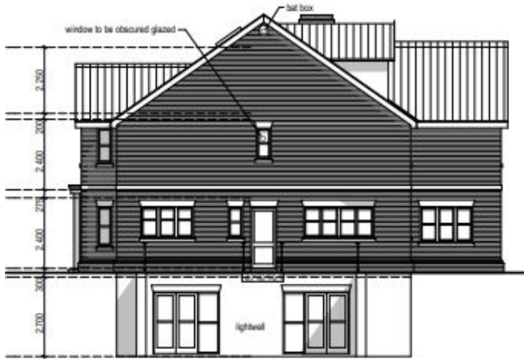
237 Hills Road house south elevation 1:100
